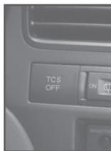
Traction Control System (TCS) Switch on Vehicle Dash
