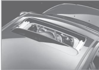
Section of a vehicle's roof that opens, either manually or motorized, as desired, to introduce sunlight or additional airflow into the passenger compartment.
